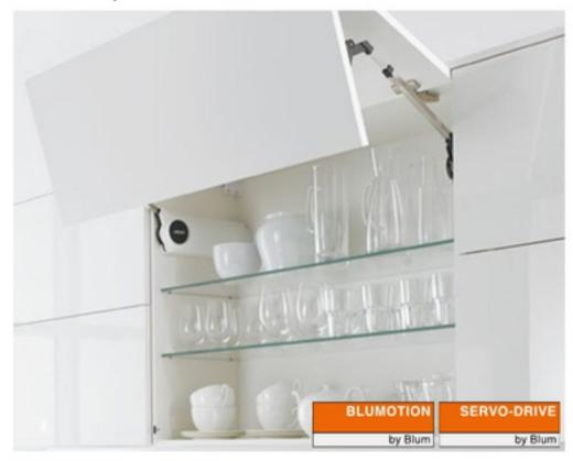
The AVENTOS HF has a two-part front that folds together in the centre when opening. The bi-fold lift system is ideal for higher wall cabinets with large fronts because the handle remains easy to reach in any position. AVENTOS HF can also be used with fronts of different heights.
